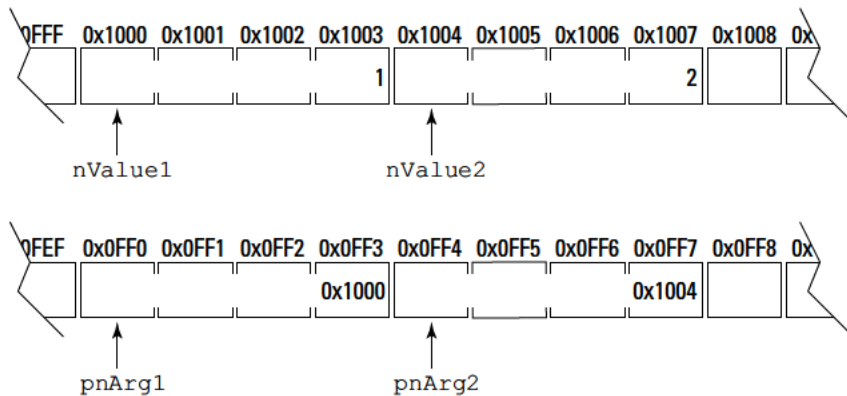
Figure 17-5: The content of memory after the call to fn ( int* , int* ).
