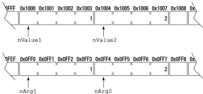
Figure 17-3: A possible layout of memory immedi- ately after entering the function fn(int, int).
